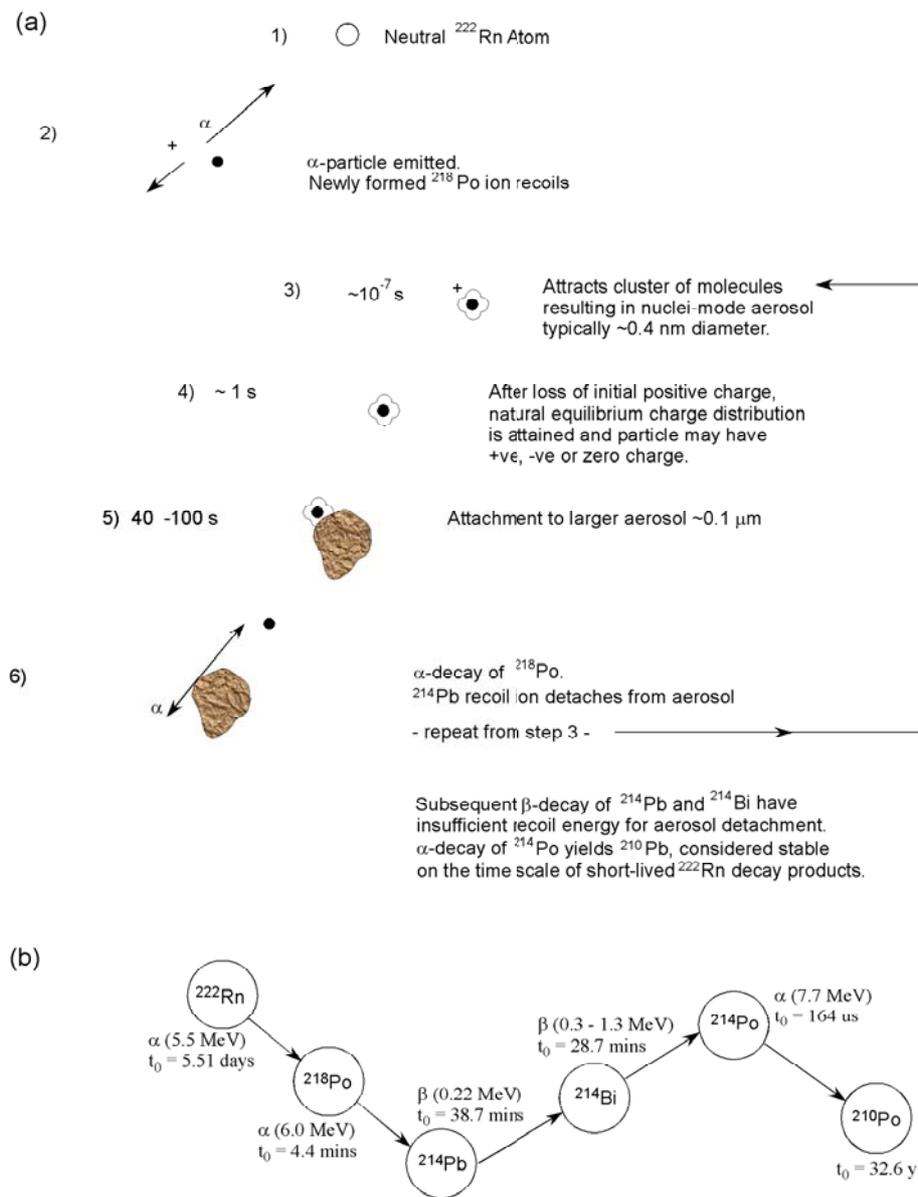
Figure 1. (a) Growth of  $^{222}\text{Rn}$  decay product aerosols (b)  $^{222}\text{Rn}$  short-lived radionuclide decay chain
