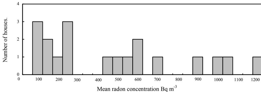
**Figure 7.** Variation in radon levels in a road of 19 similarly constructed houses in Street, Somerset.
