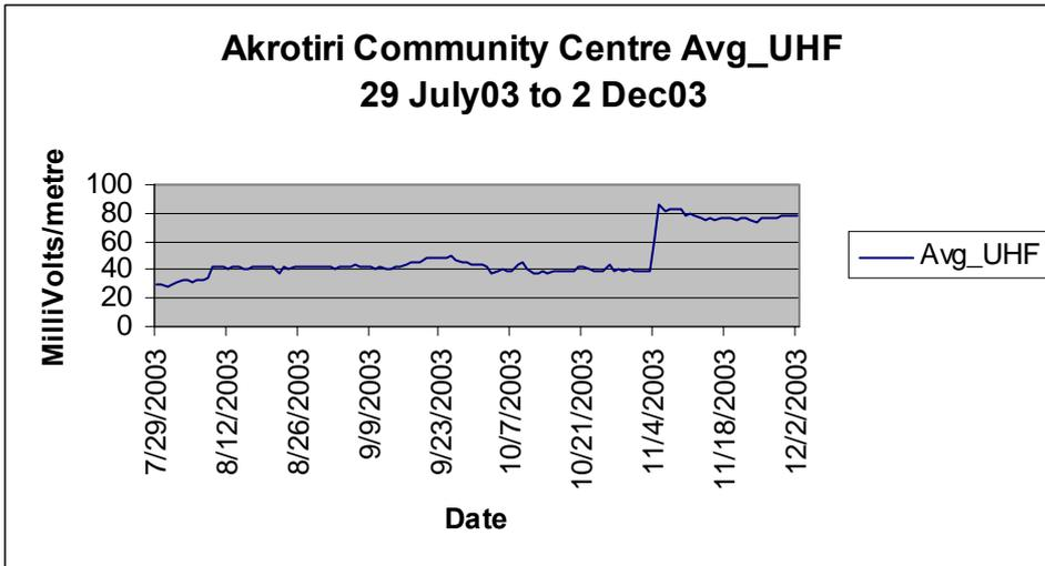
*Note the sudden increase in UHF signal on transfer to the Bank. This is because the site was some 100 metres nearer the cell-phone mast.*
