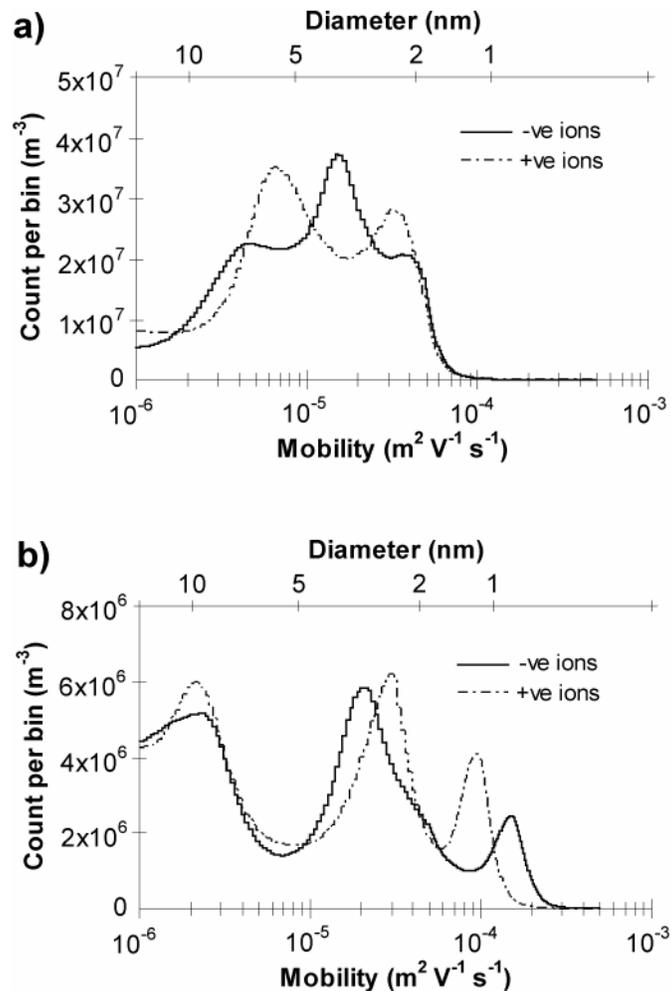
Figure 2. ACIMS mobility spectra obtained during candle burning a) with flame shielded from the fan by a lamp chimney, b) with the fan pointing away from the measurement devices.
