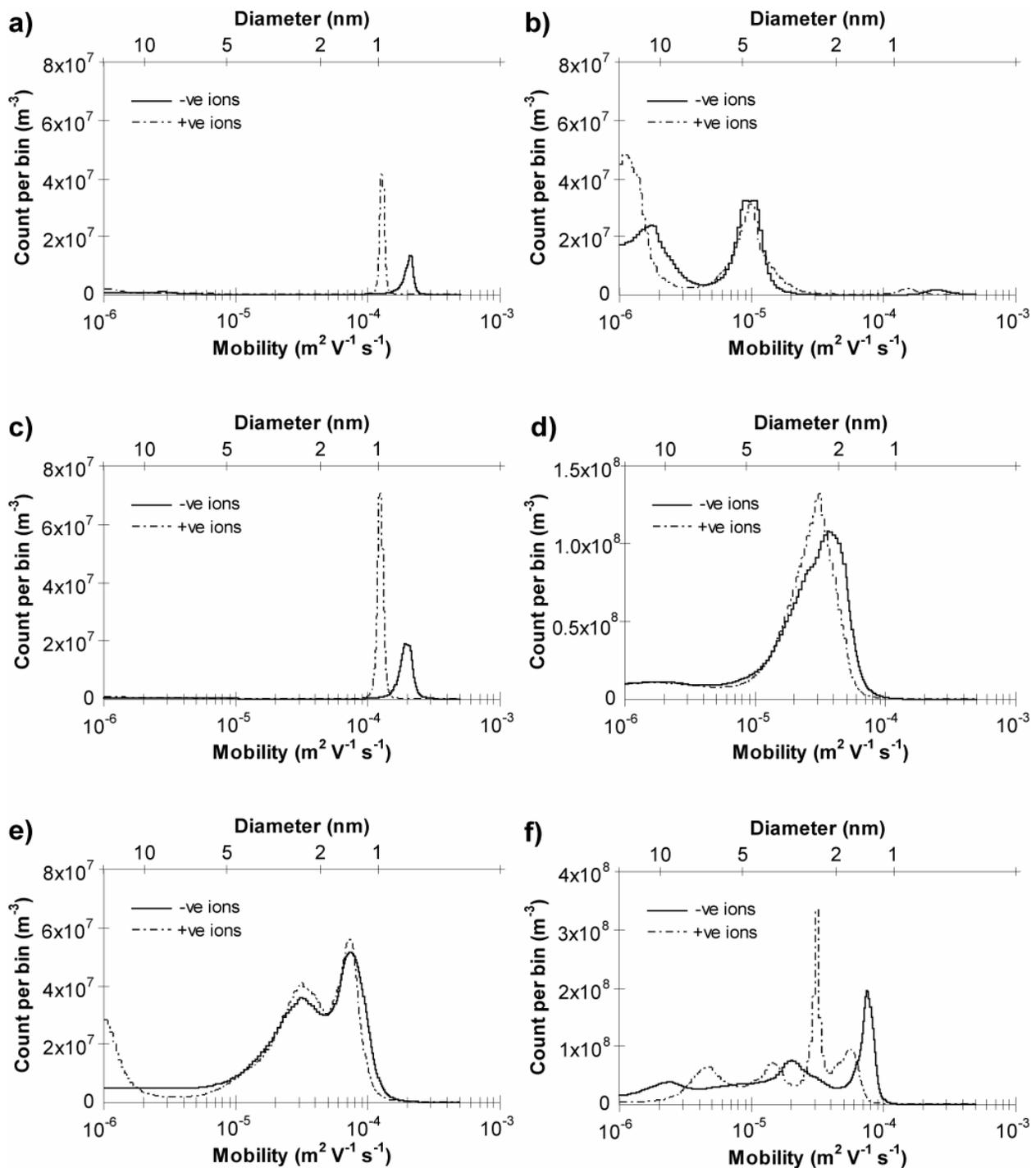
Figure 1. ACIMS mobility spectra obtained a) before lighting candle, b) during candle burning, c) several hours after candle extinguished (all on Jun 1 2005) and d), e), f) during candle burning with fan on Jul 29 2004, Jun 7 2005 and Jun 10 2005 respectively.
