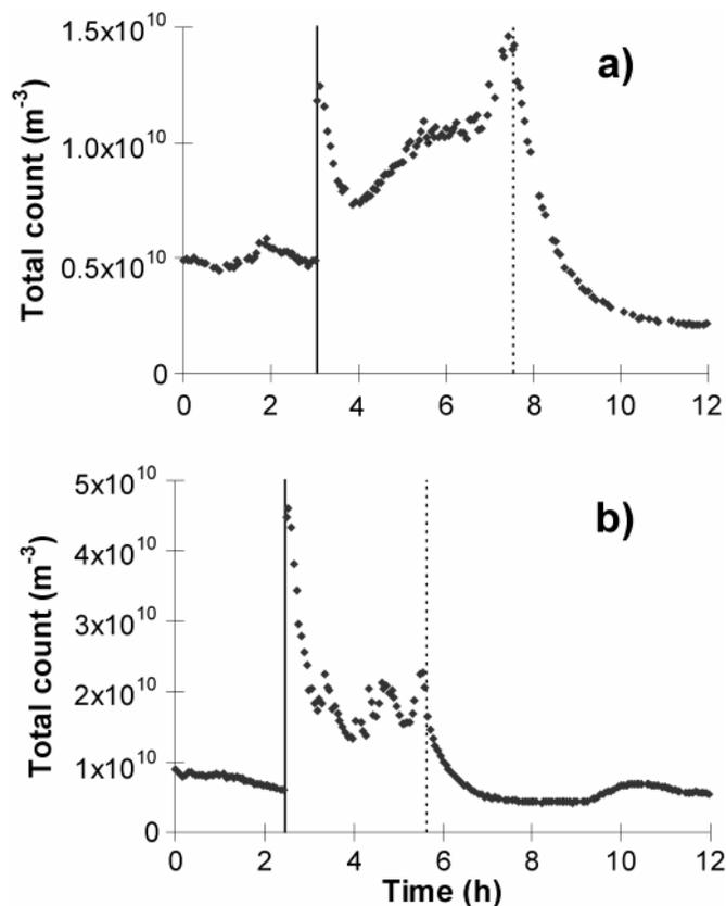
Figure 5. Aerosol counts obtained from single runs on the SMPS+C during a) candle burning on Jun 1 2005, and b) candle burning with fan on Jun 10 2006. The solid vertical lines represent candle lighting and the broken vertical lines when the candle was extinguished.
