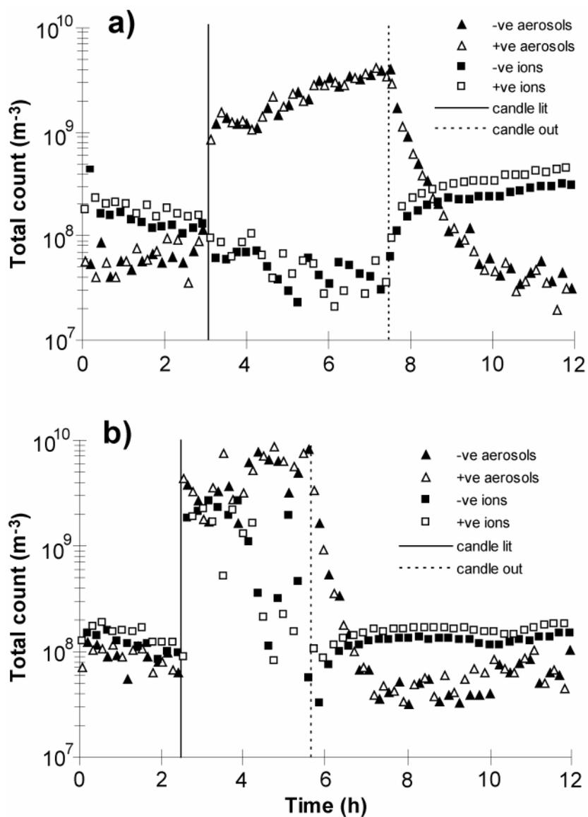
Figure 4. Small-ion and charged nano-aerosol counts obtained from single runs on the ACIMS during a) candle burning on Jun 1 2005, and b) candle burning with fan on Jun 10 2005.
