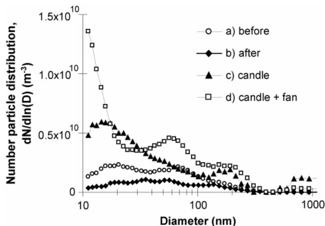
Figure 3. SMPS+C size distributions in the range 10-1000 nm. Data taken from individual runs on Jun 1 2005 (curves a to c) and Jun 10 2005 (curve d).
